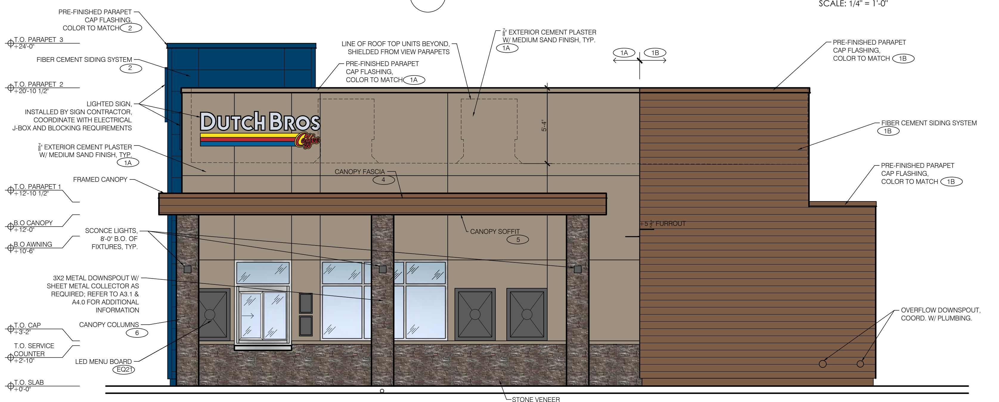
2 SOUTH ELEVATION - WALK-UP WINDOW SCALE: 1/4" = 1'-0"
